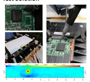
The APREL EMS (Electromagnetic Susceptibility) & SCA (Side Channel Attack) application is designed to support the design, development, and assessment of ICs, mobile devices, automotive components, and electronic assemblies for vulnerabilities of cryptographic attacks. This solution enables testing the security of circuits against radio frequency side-channel attacks.
