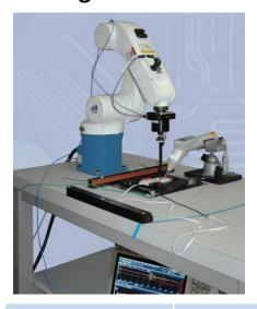
The **EM-ISight-ESD** is a fully integrated test system designed to measure test subjects exposed to an electrostatic discharge (ESD) source. As an industry-first solution, it enables real-time measurement of certified ESD events across frequency, time, integrated, and spatial fields on devices subjected to controlled ESD events.
